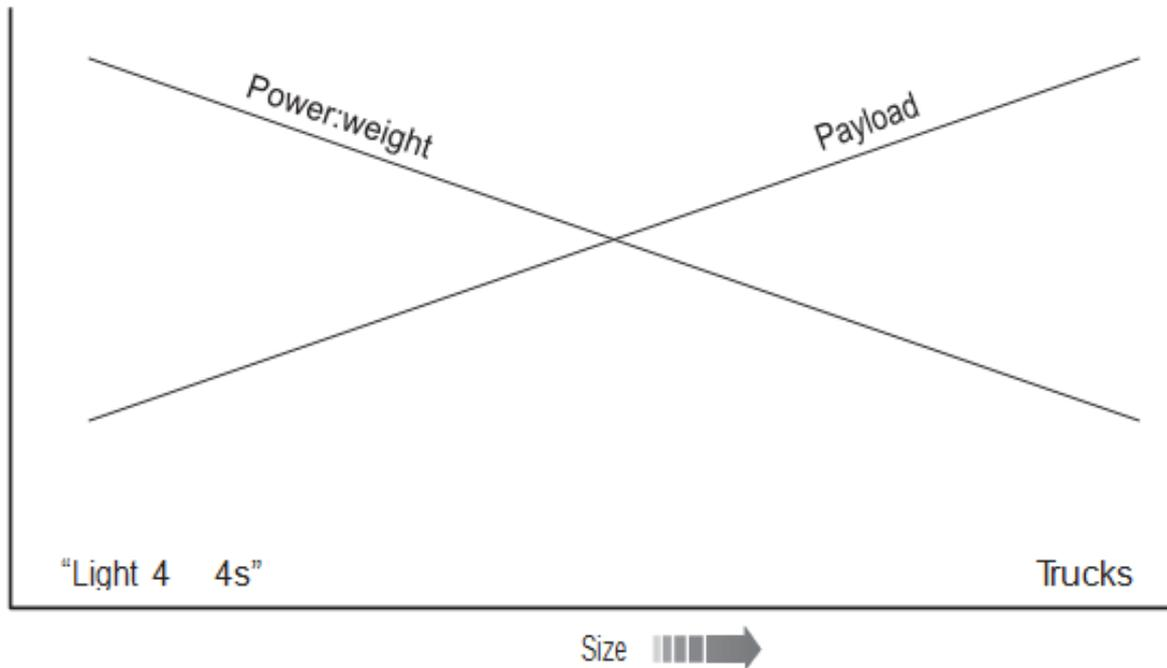
*Figure 28.6 The size trade-offs: power:weight ratio and payload*
