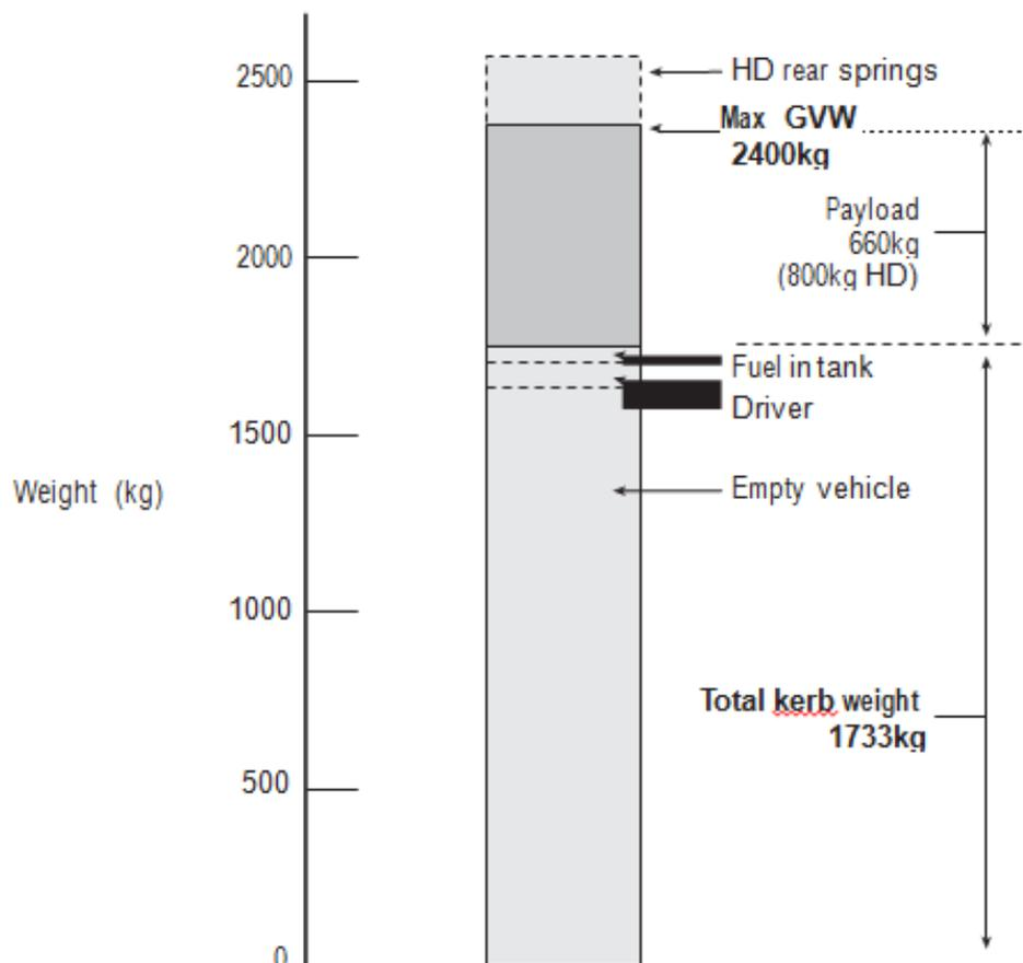
Figure 28.1 How a vehicle's GVW (gross vehicle weight) is made up. Never exceed it by adding too much payload. Figures shown are for Defender 90
