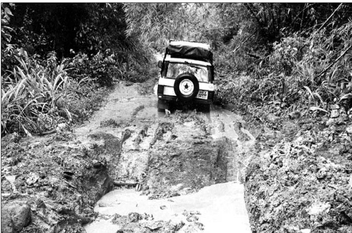
*Figure 28.8 A 4 x 4 is best. Here, as with rock crawling or steep washouts, low-range gears are virtually essential (© Tom Sheppard)*
