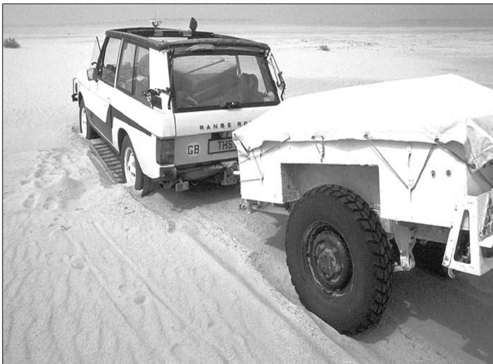
*Figure 28.5 Classic example of a fuel-carrier trailer off-loading the main vehicle. Note also how the under-tyred tug has bogged whereas the lightly laden trailer on larger tyres at low pressures rides over the soft sand (© Tom Sheppard)*
