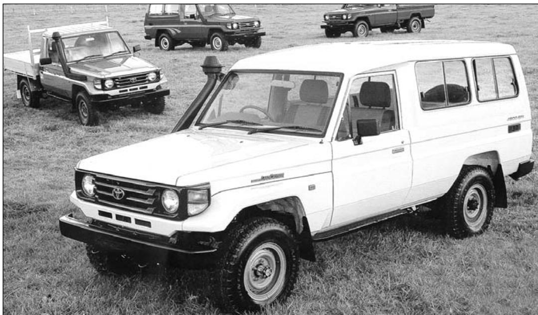
*Figure 28.9 Classic robust simplicity – the Australian spec Toyota Type 78 even comes with long-range fuel tanks as standard. This one has coil springs at the front. Never imported into UK, earlier all-leaf-sprung Type 75 in diesel form is highly valued in continental Europe for expedition work (© Tom Sheppard)*
