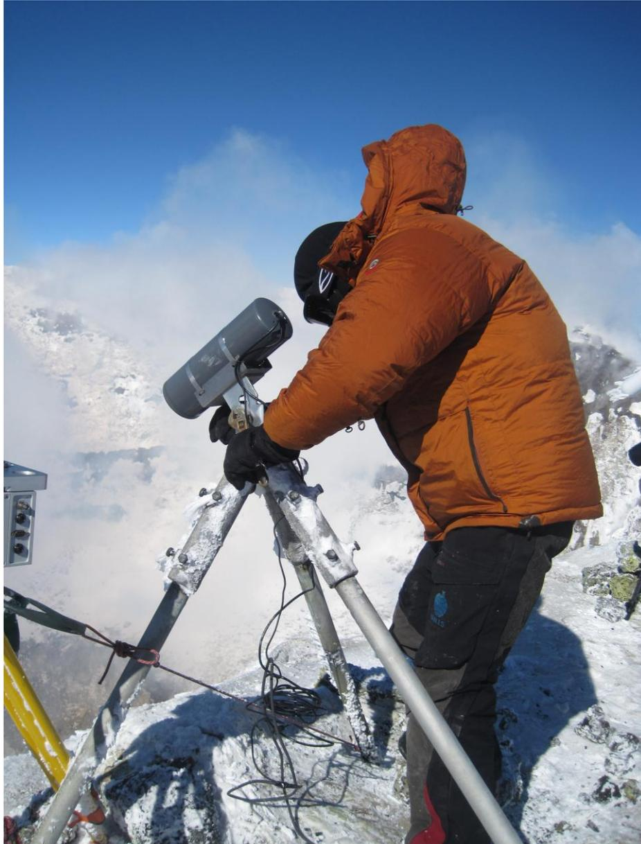
The thermal imaging camera helps observe heat from the volcano. On Erebus it helps measure the variation in the level of the lava lake. It can also help understand the changes in heat emitted from the lava plume.
