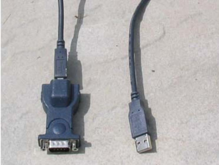
*Figure 11-2 Serial - RS232 9 pin male to USB converter. The RS232 serial connector is shown on the left and the USB connector is shown on the right. The RS232 connector receives the female GPS connector and transfers the data through the USB port of the PC.*
