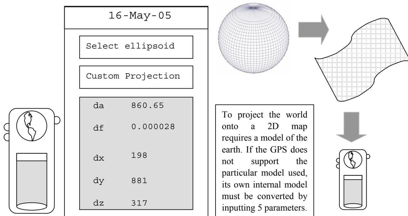
Figure 11-1: Inputting user datums into a GPS.
