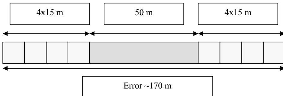
Figure 11.6a Errors generated from rectification (in X dimension using Landsat ETM+ data).
