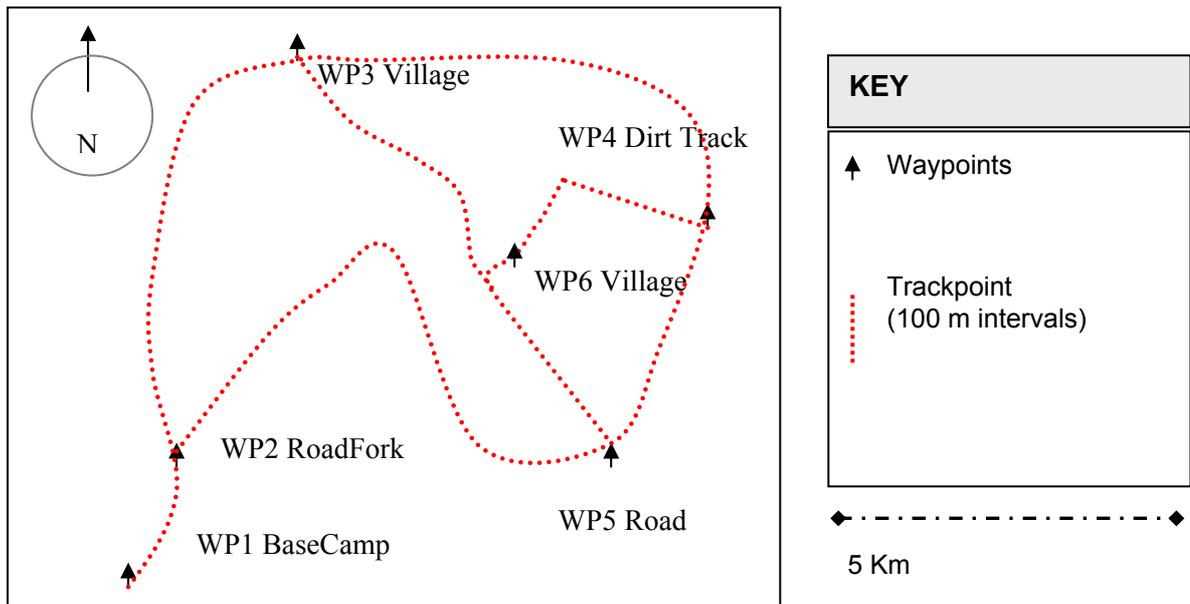
Figure 11-5 Schematic point plot of GPS Data showing road and tracks in a study area annotated with waypoints. This type of information can be displayed from the GPS screen or it can be downloaded into a Utility such as GPS Utility or downloaded and plotted into a GIS.
