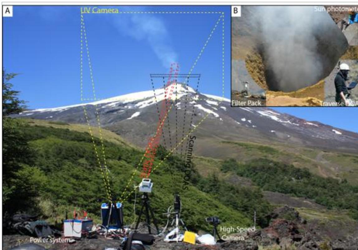
**Figure 2:** A. Typical multi-instrumental setup to monitor Villarrica degassing from Los Crateres observation site. B. Additional instrumental deployment made simultaneously at the crater rim of February 8 and 10.
