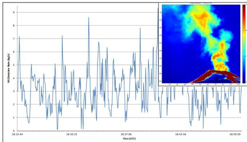
**Figure 6:**  $\text{SO}_2$  flux in kg/s vs Time. Upper right inset shows a Calibrated  $\text{SO}_2$  absorbance map showing the  $\text{SO}_2$  concentration in the volcanic plume rising from the crater.
