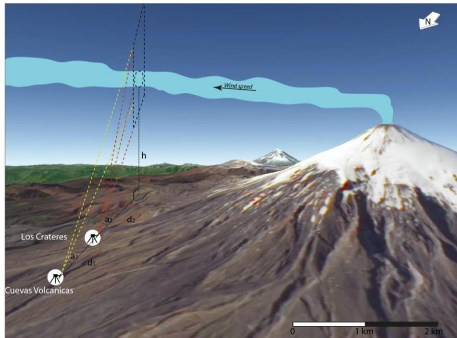
**Figure 3:** Schematic representation of the parallel scanning DOAS method used on Feb 11 where  $h$  is the plume height,  $d_1$  and  $d_2$  the distances from los crateres to cuevas volcanicas and to the plume respectively and  $a_1$  and  $a_2$  are the angle recorded by both scanning DOAS.
