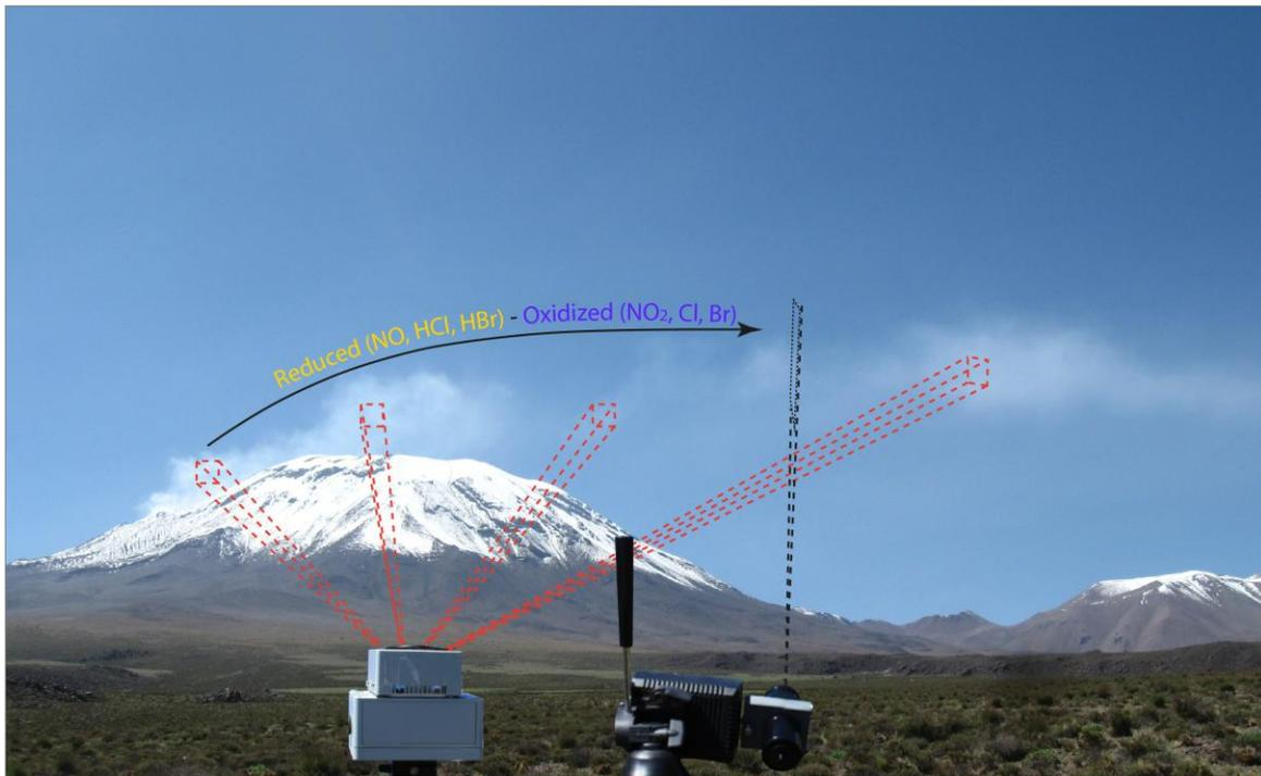
**Figure 5:** Schematic representation of the multiple static DOAS technique to study the chemical evolution of the aging plume at Lascar volcano.
