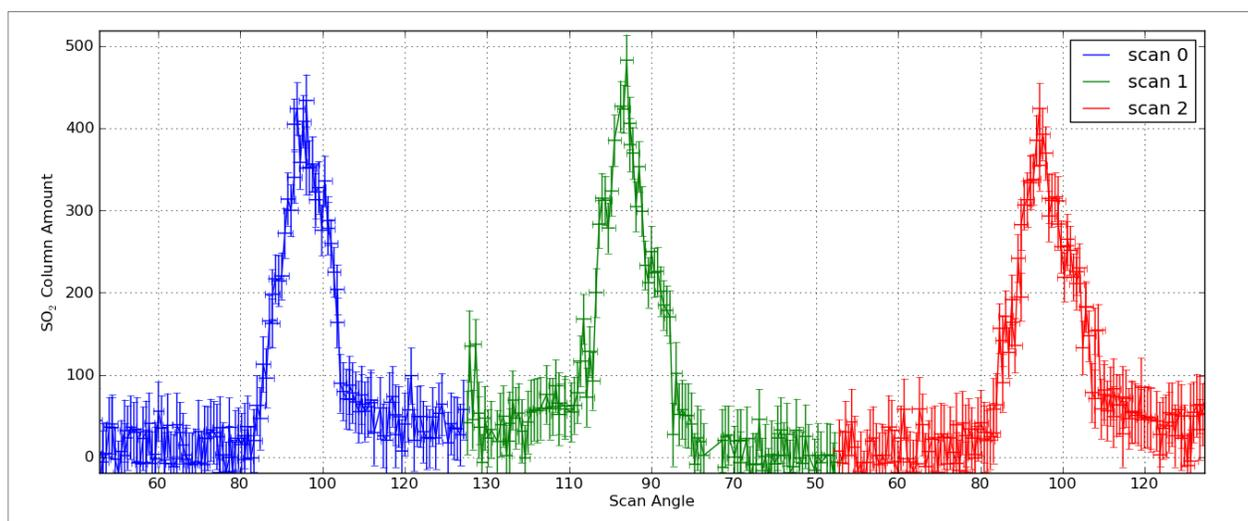
**Figure 7:** Plot of SO<sub>2</sub> column amount against scan angle from three horizontal scans of the Lascar plume.
