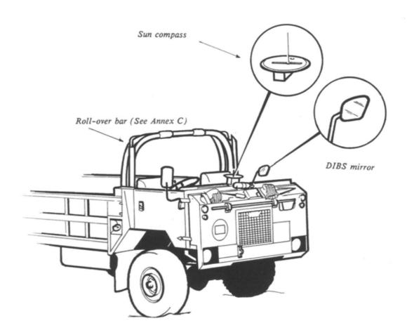
*Use and mounting of a sun compass – on any vehicle – is greatly enhanced by removal of windscreen*
