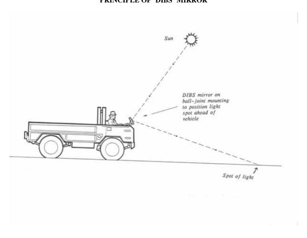
Optimum mirror to use of DIBS application is about 6in x 8in and must be flat: a convex mirror will not project a light spot.
