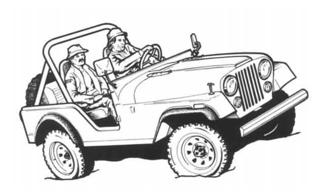
Roll-over bar shown on US 'recreation vehicle' CJ5 Jeep illustrates well the principle of fore-and-aft bracing as well as lateral strength. Installation is a wise precaution in any vehicle to be used with upper bodywork removed to aid visibility and save weight. Compare with roll-over bar shown in Anne B which, though amply strong in roll, is inadequately braced for-and-aft.
