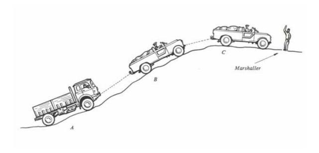
Marshaller first waves vehicle B forward till tow-rope A-B is taut; then he ensures tow-rope B-C is taut. Then, with all three vehicles' engines used and all in the best gear (low range, second gear, in this case in order not to over-torque the loose ground), he drops his arm and on the signal all three drivers let in their clutch. It is essential that all the drivers take their 'go' signal and 'stop' *instructions from one man – the marshaller.*
