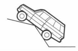
A good ramp angle is important and results from a combination of large wheels and a shortish wheelbase.
