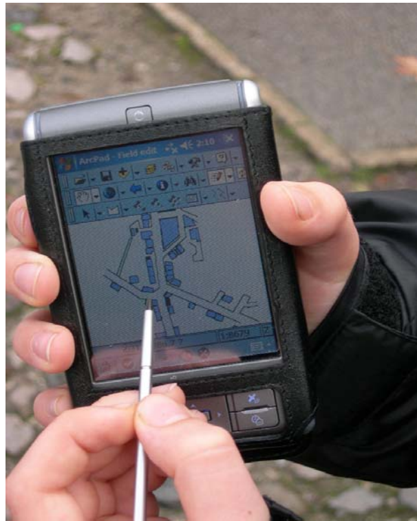
Gathering data in the field using a Loox N520 with ArcPad software
