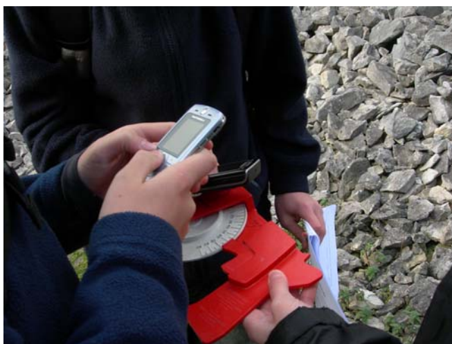
Slope data being Bluetooth transferred to another group mobile. Data also forwarded to School using SMS for analysis in class.
